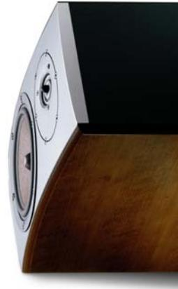
Also, the planar design gives optimum working conditions, i.e. a minimum of diffractions, for the asymmetrical placed tweeter. By choosing the asymmetrical design, no distances from cabinet top and sides to the tweeter are identical and thus edge reflections do not accumulate. The result is a crystal clear treble reproduction – which is essential in order to benefit from the extended treble contents of the new multi channel sound formats.
