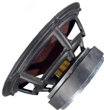
The basket is made of magnesium giving several benefits: First of all it makes it possible to create a very open basket – even behind the spider – thus ensuring high airflow at low frequencies, avoiding reflections at high frequencies and preventing under-/overpressure causing mechanical losses.
