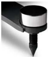
The D 4FS can be placed either by using the adjustable spikes securing a good mechanical coupling to the floor independent of floor materials or, if you prefer to decouple it from the floor, by using the enclosed rubber absorbers. The design and choice of material for the rubber absorbers (PUR 80 Shore A) was made to match exactly the D 4 speakers.
